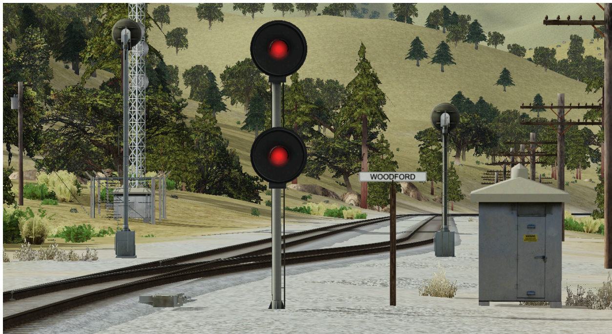
A home signal showing "stop" with a control point sign (and electronic switch machine on the bottom left).
