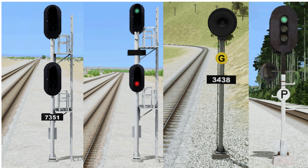
Examples of intermediate signals, from left to right: numberplate with numbers, numberplate without numbers, a grade plate (and numberplate with numbers), and a permissive plate.
